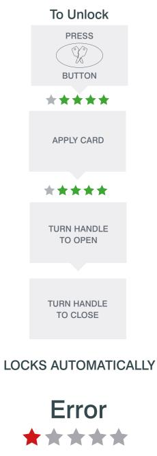
Errors will time-out after 4 seconds. Unfinished instructions will time-out after 4 seconds. Always wait for LED lights to finish before pressing next key.
