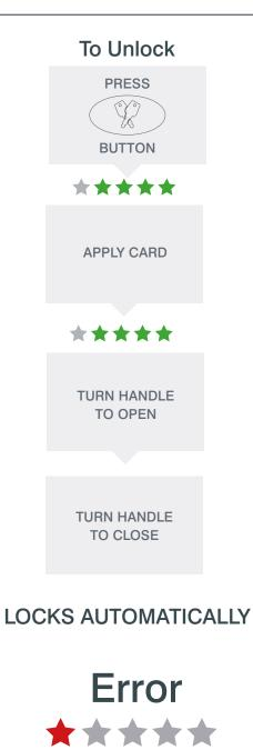
Errors will time-out after 4 seconds. Unfinished instructions will time-out after 4 seconds. Always wait for LED lights to finish before pressing next key.
